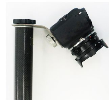
Figure 4. Camera holder for terrestrial photogrammetry.
