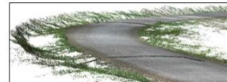
Point cloud (an example of photogrammetric point cloud with cross profiles surveyed geodetically).
