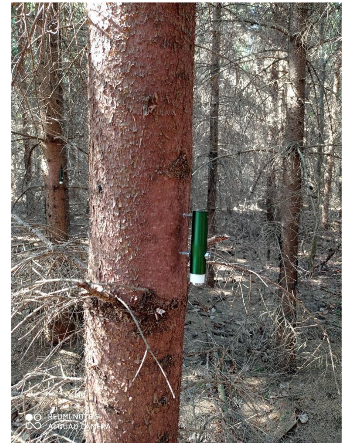
Fig. 1: The automatic point dendrometer model D2 installed in the unthinned control plot.
