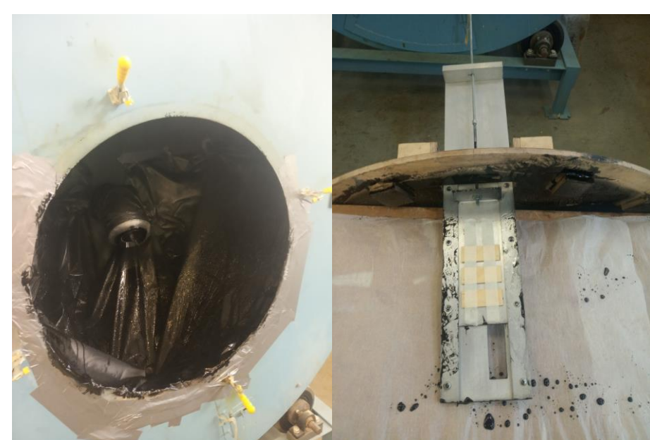
Fig. 1: Adhesive application to the specimens in rotary blender with spinning disc atomizer.
