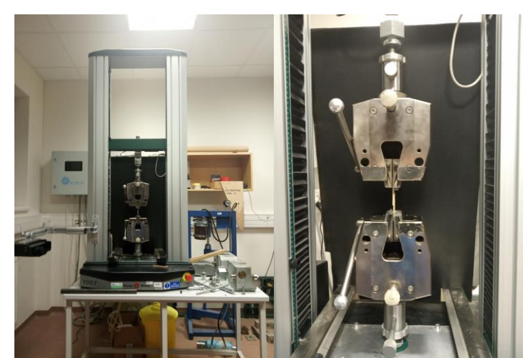
Fig. 4: Testing specimens by Tinius Olsen 10ST (Redhill, UK)
