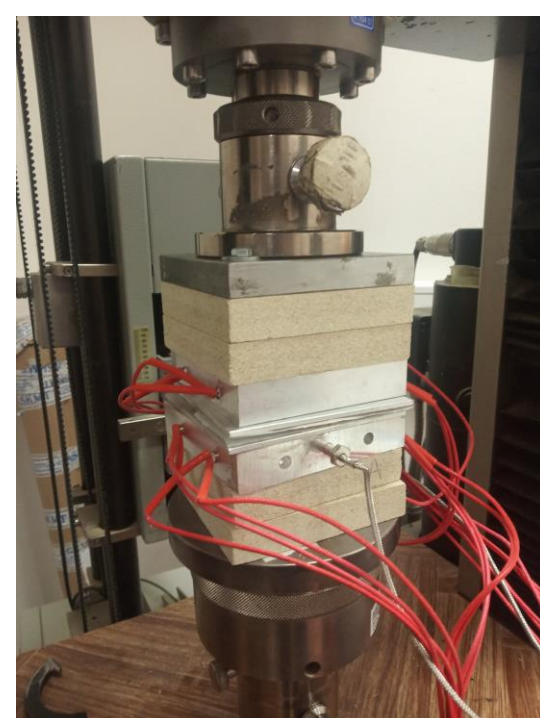
Fig. 2: Pressing specimens by universal testing machine Zwick Z050 (Zwick Roell, Ulm, Deutschland)
