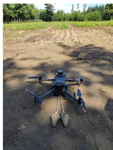
Biodegradable seed capsules mounted on UAV
