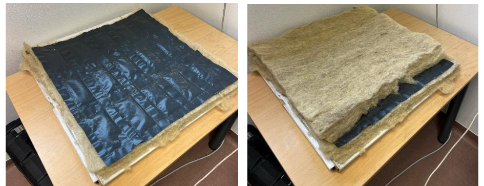
Figure 2: To produce macrocapsules, a PE foil with a thickness of 0.2 mm was used. The macrocapsules had dimensions of 200x130 mm and were filled with 50 ml of paraffin. The individual macrocapsules were then joined by welding to form a uniform layer and thus a homogeneous structure was achieved.
