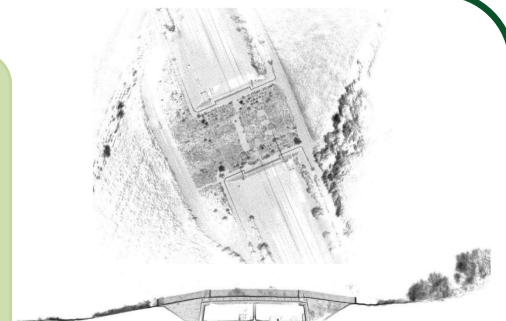
Figure 8. 3D model of the surface and vegetation of the green bridge
