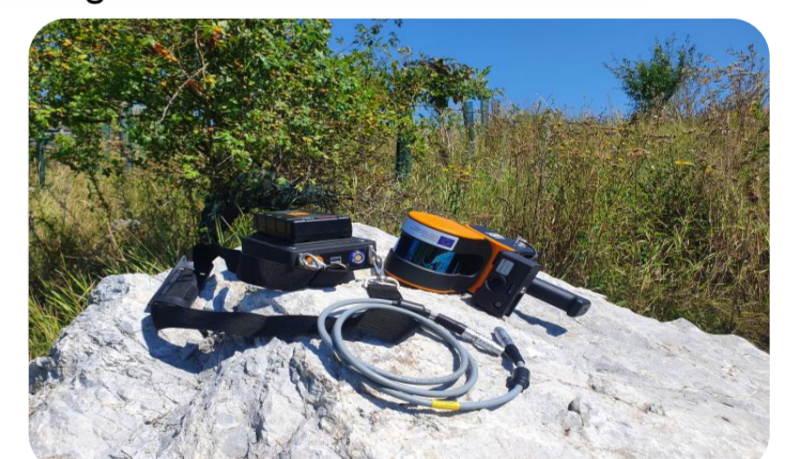
Figure 6. Hand-held ZEB HORIZON 3D scanner
