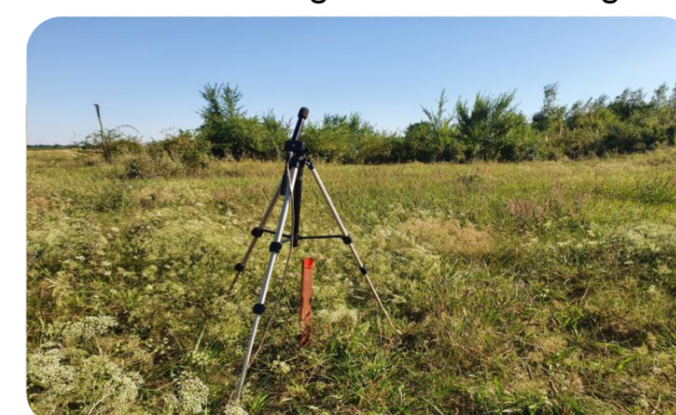
Figure 5. Measurement of traffic noise with the NTI Acoustilyzer AL1
