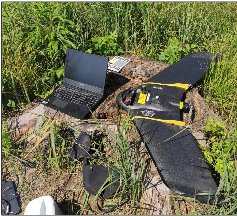
Figure 1 Unmanned aerial vehicle eBee SenseFly plus
