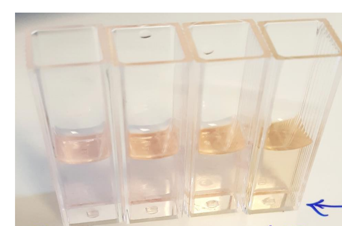
Fig. 4: Tannase assay – calibration showed limited range (absorbance) response at proposed wavelength 520 nm
