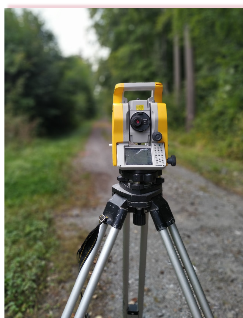
Figure 2. Total station Trimble M3 used for measuring spatial coordinates X,Y,Z of reference crosses
