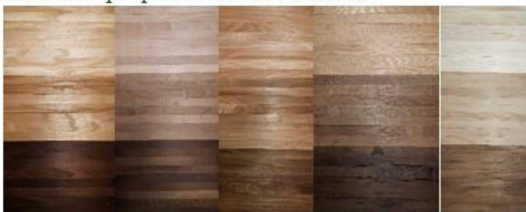
Fig 1. the thermally treated samples of ash, beech, larch, oak, spruce (from left to right) for untreated, 180°C and 220°C treated groups (from up to bottom)
