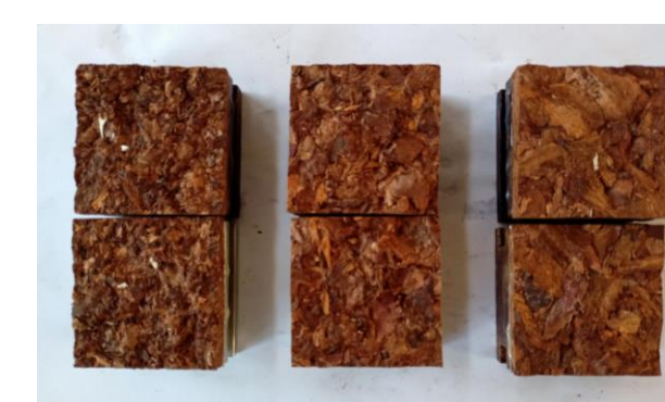
Fig. 19: failure samples from spruce bark bonded with 5% UF resin after IB testing.
