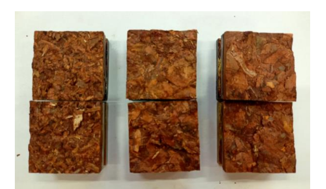
Fig. 20: failure samples from pine bark bonded with 5% UF resin after IB testing.
