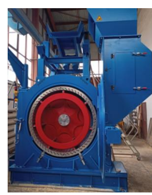
Fig. 2: desintegration flaker MRZ/MSF 1400
