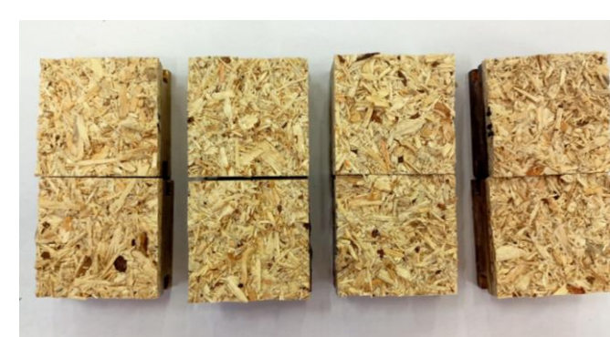
Fig. 18: failure reference samples bonded with 5% and 7% UF resin after IB testing.
